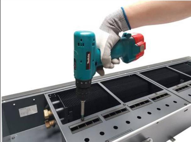
Fig. 8: Loosening screws in the cover
